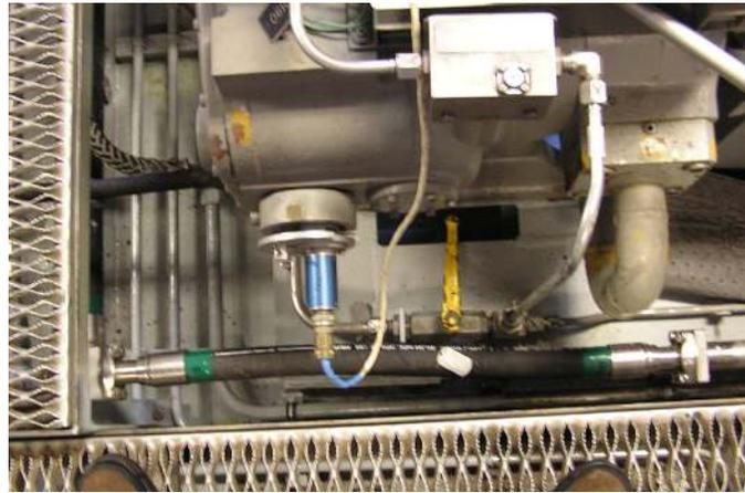
Figure 5: flexible hydraulic hose
