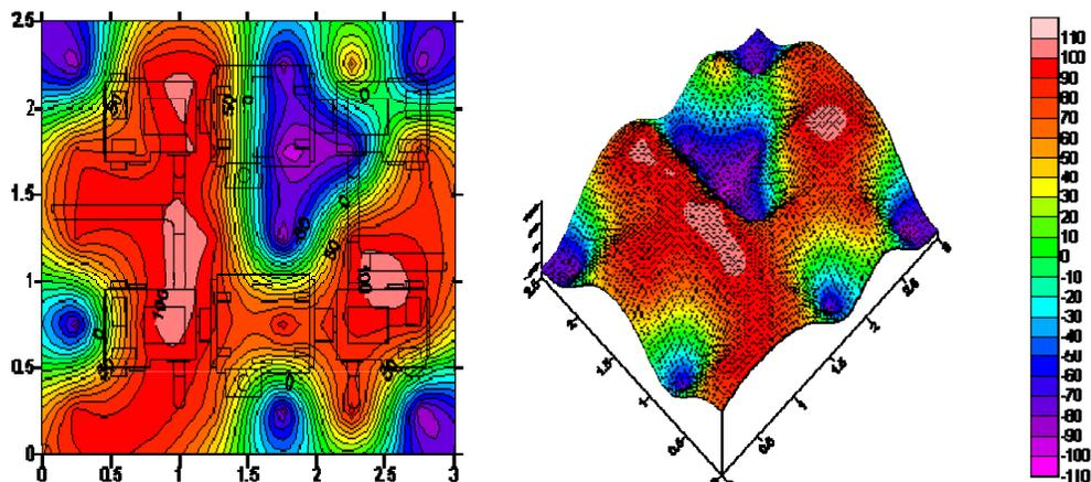
Figure 1: JEL hydraulic pumps 400 Hz Sound Intensity Plot
