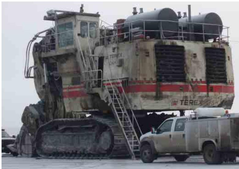
**Figure 6:** Terex RH200 engine exhaust silencer installation.
